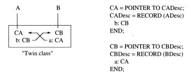
Fig. 8.13 Resolving multiple inheritance with a twin class
