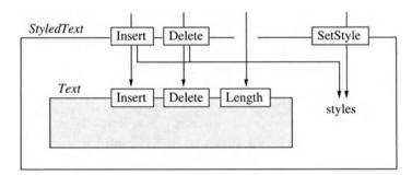
Fig. 7.7 StyledText as a new layer around Text
