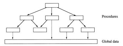
Fig. 1.8 Calling graph of procedures working on a set of global data
