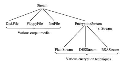
**Fig. 8.7** Field *s* of *EncryptionStream* can contain *DiskFile*, *FloppyFile* or *NetFile*
