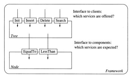
Fig. 7.1 Interfaces of a class to its clients and components
