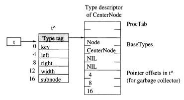
**Fig. A.12.1** A variable *t* of type *CenterTree*, the record *t*^ of type *CenterNode*, and its type descriptor
