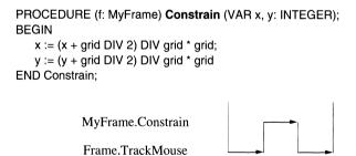
**Fig. 8.20** Adding behavior to an inherited method by overriding a hook method
